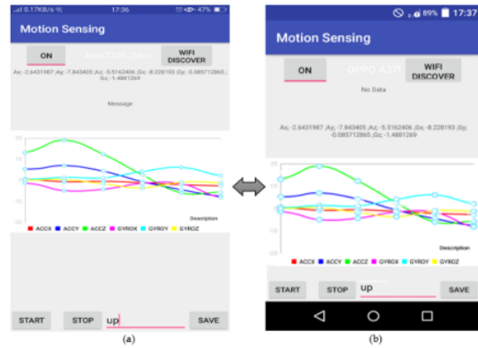
Fig. 6. Screenshots display of up arm motion (a) Transmitter (b) Receiver
