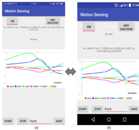
Fig. 4. Screenshots display of forward arm motion (a) Transmitter (b) Receiver
